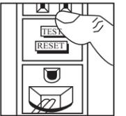
(c) If you installed your GFCI using step 7B, plug a lamp or radio into surrounding receptacles to see which one(s), in addition to the GFCI, lost power when you pressed the TEST button. Do Not plug life saving devices into any of the receptacles that lost power. Place a "GFCI PROTECTED OUTLET" sticker on every receptacle that lost power. Then press the RESET button to reset the GFCI.
