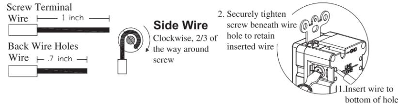
**Connect the LINE cable wires to the LINE terminals:**
