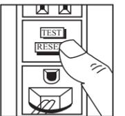
(d) Press the TEST button (then RESET button) every month to assure proper operation. If the GFCI can not be reset, then it must be replaced.
