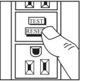
(b) Press the TEST button in order to trip the device. This should stop the flow of electricity, making the radio or lamp shut OFF. The Green LED load side voltage indicator will turn OFF. Note that the RESET button will pop-out. If the power stays ON, go to Troubleshooting. If the power goes OFF, you have installed the GFCI receptacle correctly. To restore power, press the RESET button.
